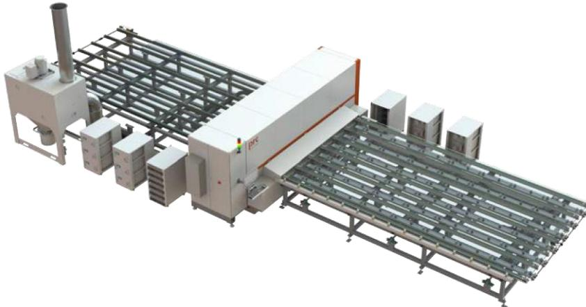
**Bird friendly:** can apply laser markings of various transparency on windows of up to 6 m x 3.3 m size
